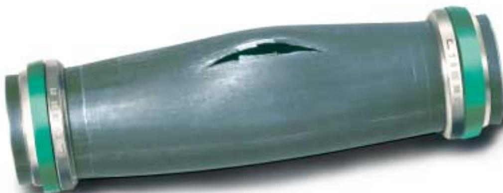
*Destructive testing with 28x2 carbon steel tube
