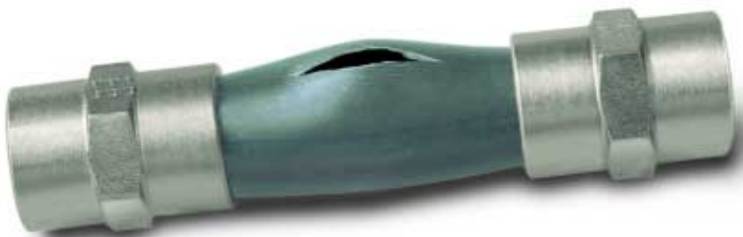
Destructive testing with 22x2 carbon steel tube The tube burst at 800 bar without any leaks or sweating from the sealing points.
